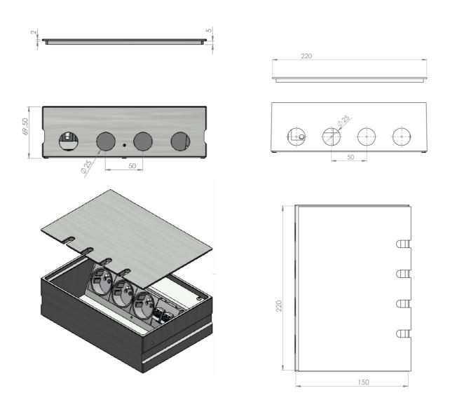
Attention!: The lid is partially (5 mm) insered into the box and 2mm extends (on height) over the box.
